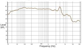
Frequency response measurement with transducer mounted in a 20 liter vented enclosure tuned to 65Hz
