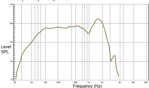
Frequency response measurement with transducer mounted in a 180 liter vented enclosure tuned to 35Hz
