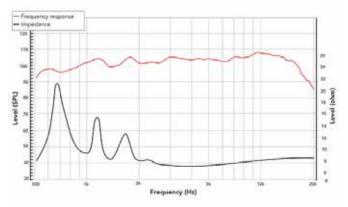
Frequency response measured on IAC baffle
