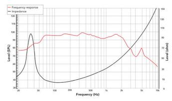
Frequency response measured on IAC baffle
